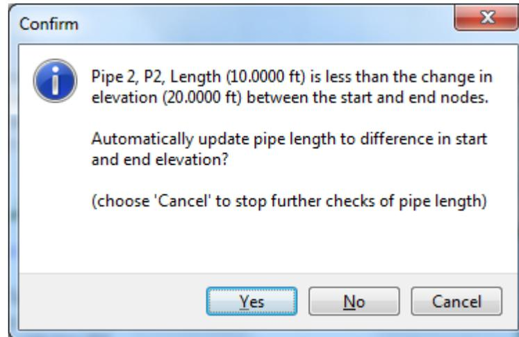
Where pipe lengths are not sufficient to span the difference in node elevations, these pipes will be identified and the user will be asked to confirm an update for each pipe. The pipe length can automatically be set to the difference in start and end elevations of the pipe.
