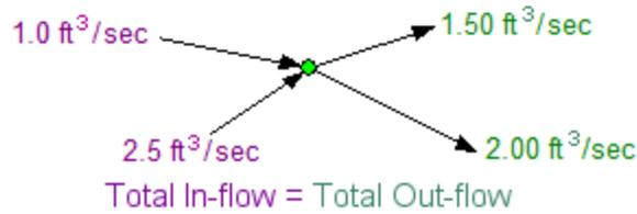
Figure 92 Flow balance at a join point
