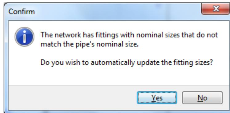
If the nominal pipe size does not match some of the fitting sizes associated with the pipe, then the option to update the fitting sizes should normally be accepted. This will update the fitting sizes and the fitting 'K' values so that the fitting pressure losses will be calculated correctly.
