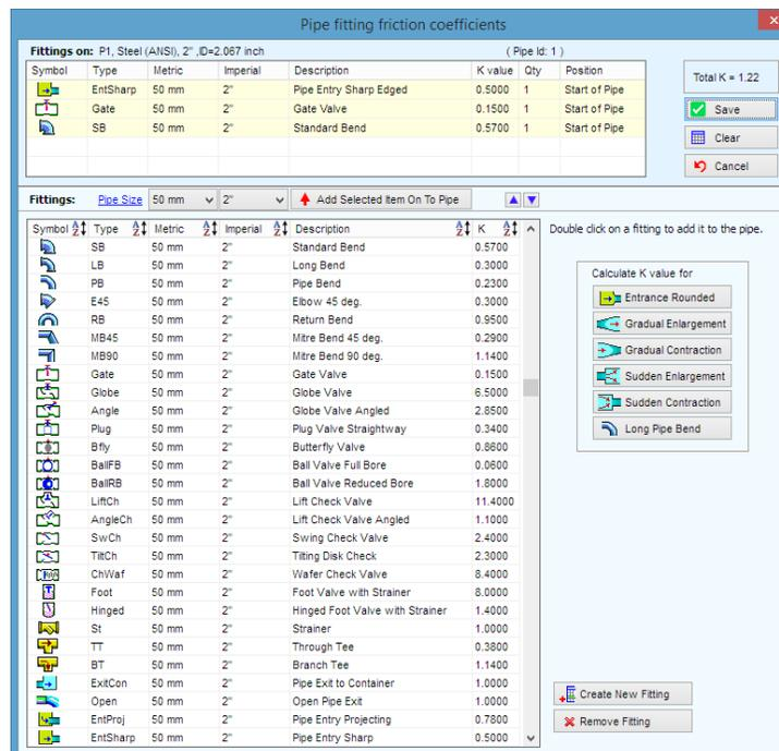
Figure 54 Pipe fitting friction coefficients database
