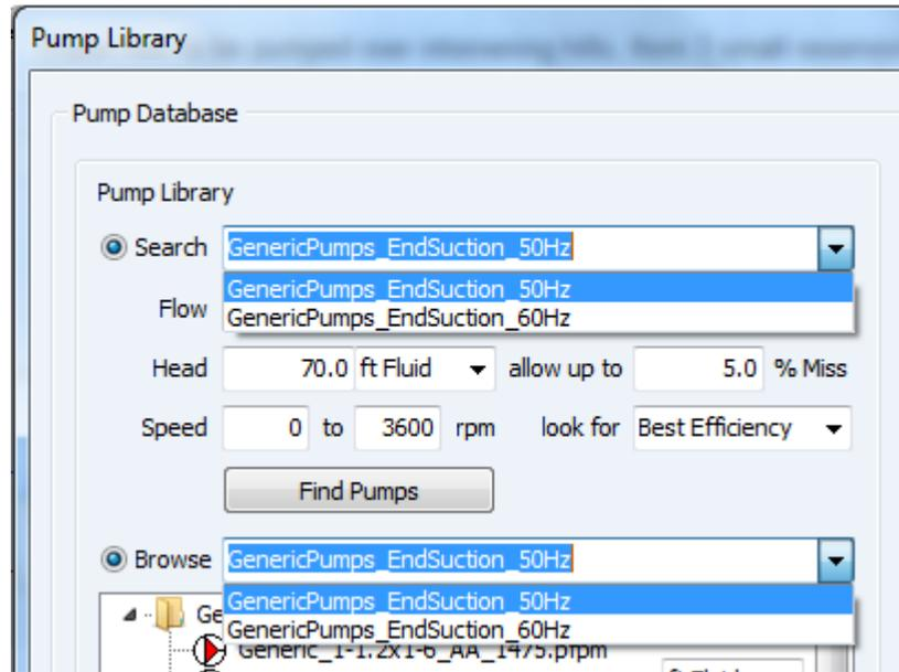
The example pumps can be loaded and used to see the results that are produced by using different pump operating data. This data is provided solely as example data and is not related to any specific pump manufacturer. When adding further pump data to the pump database, we recommend that a new folder is created for each pump manufacturer. The pumps can then be organized and saved in named folders.
