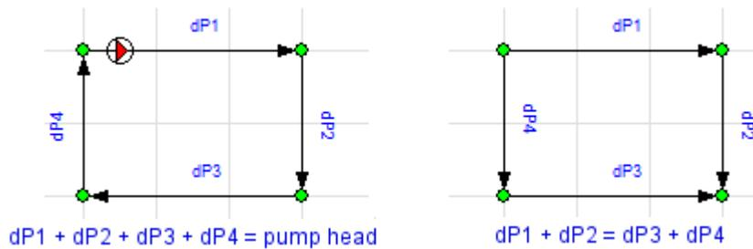
Figure 93 Pressure balance around a loop
