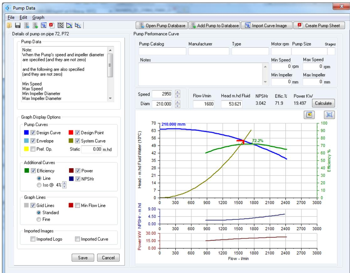
Figure 69 Pump Graph with NPSHr and Power
