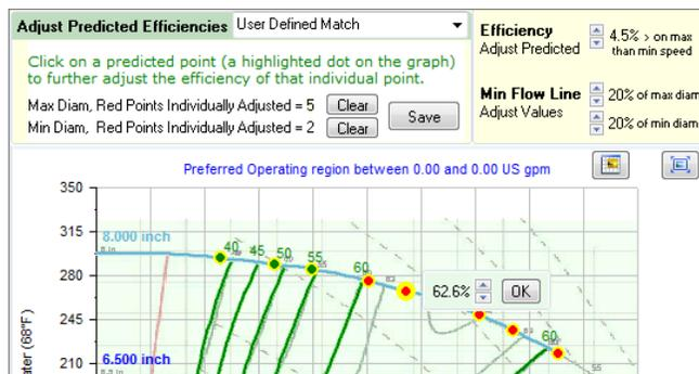
To adjust an individual efficiency point, click on a 'Green' point on the performance curves and use the up/down adjustment to set the efficiency value for the point.
