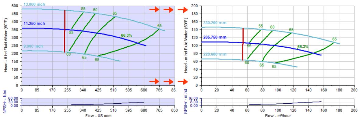
Both the performance curve and the NPSHr curve can be shown in the pump graph window.
