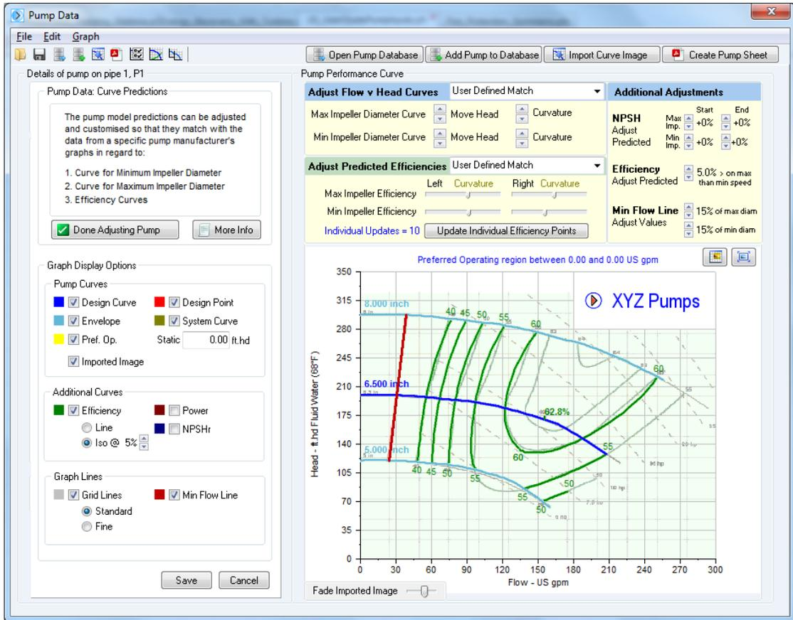
Figure 72 Adjusted Pump Model
