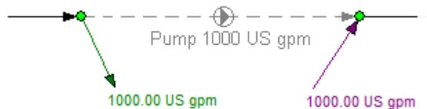
**Figure 98 Fixed Flow Rate Pump replacement**
