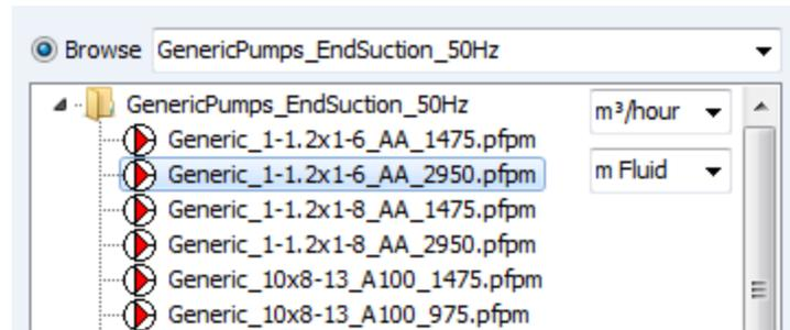
Once a folder is selected, the pumps within the chosen pump library folder are displayed in the Browse List, where the user can click on a pump to show its corresponding pump performance graph.
