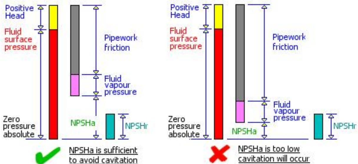
In a system where the fluid needs to be lifted to the pump inlet, the negative head reduces the motive force to move the fluid to the pump. In these instances it is essential to size the supply pipe work and isolating valves generously so that high frictional losses do not reduce the NPSHa below the NPSHr.
