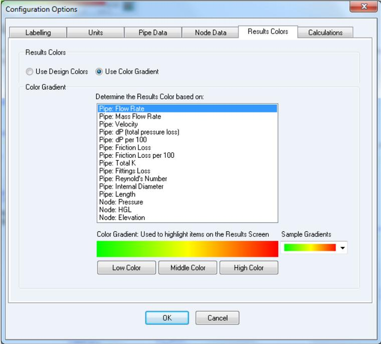
Figure 43 Configuration Options – Results Colors Tab
