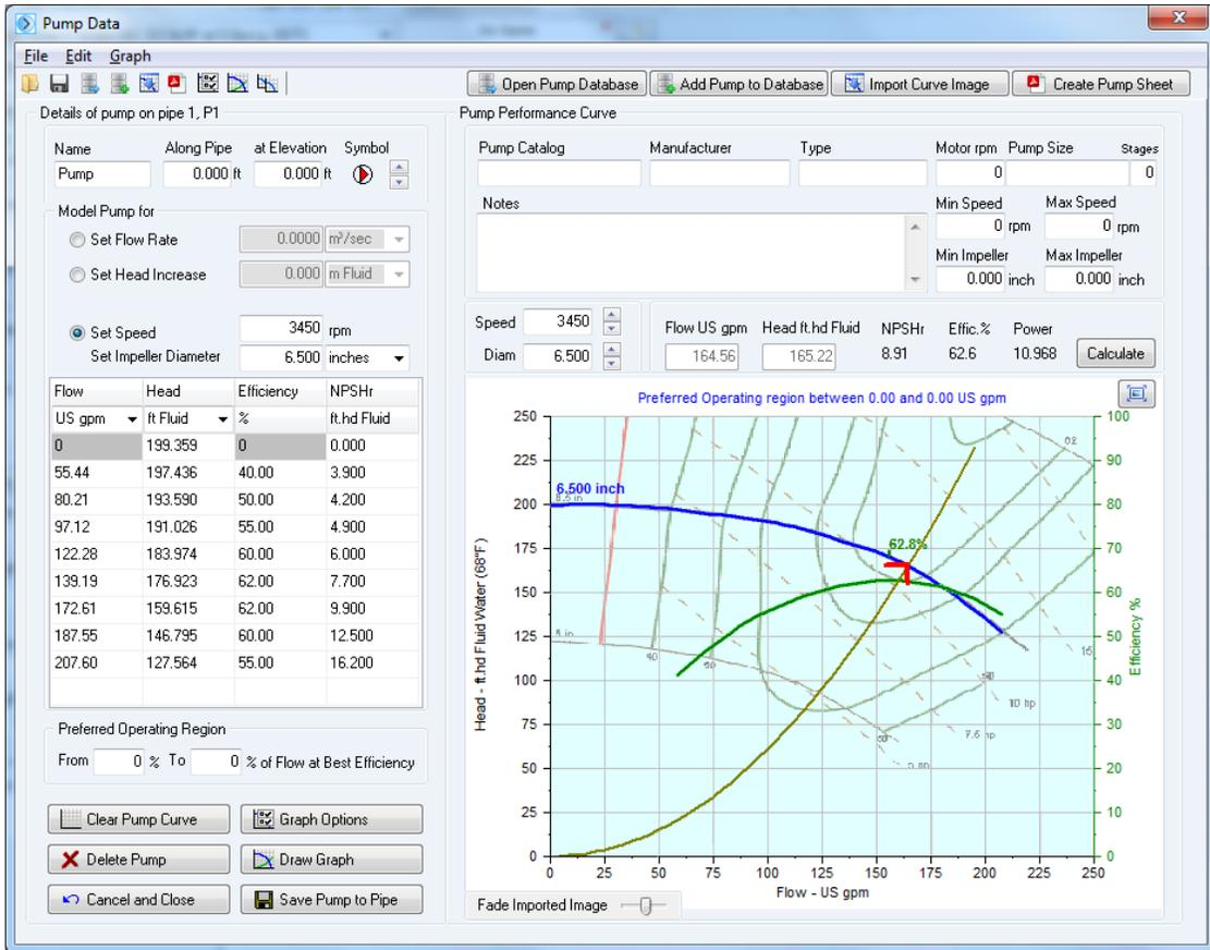
Figure 70 Simple Pump Graph from imported points
