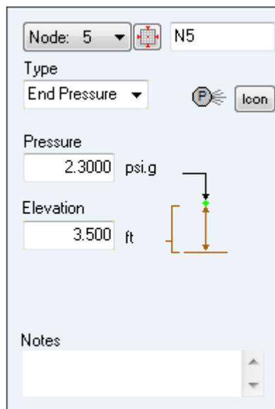
The screenshot shows the Node pane for Node 5 (N5). The Type is set to End Pressure. The Pressure is 2.3000 psi.g and the Elevation is 3.500 ft. A small diagram to the right shows a pipe with a demand pressure symbol at its end. The Notes field is empty.
