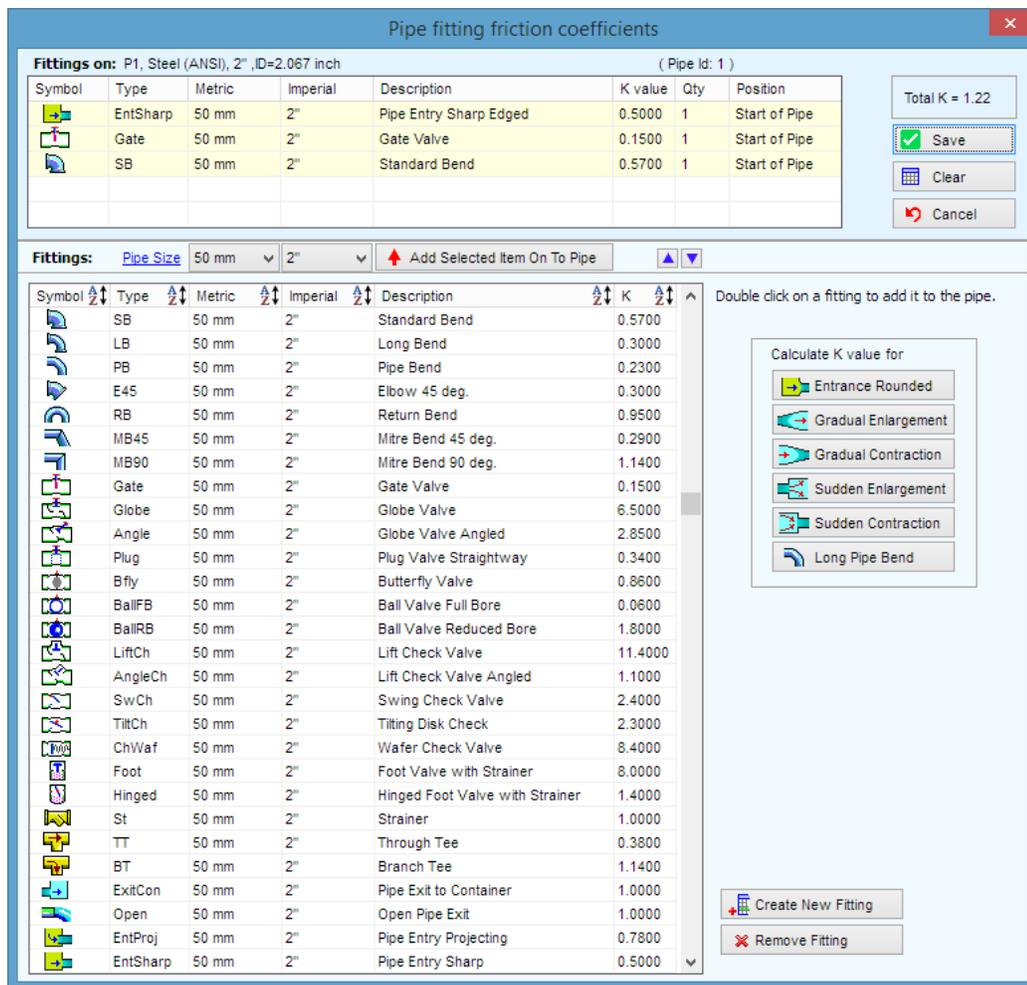
**Figure 40 Pipe fitting friction coefficients**
