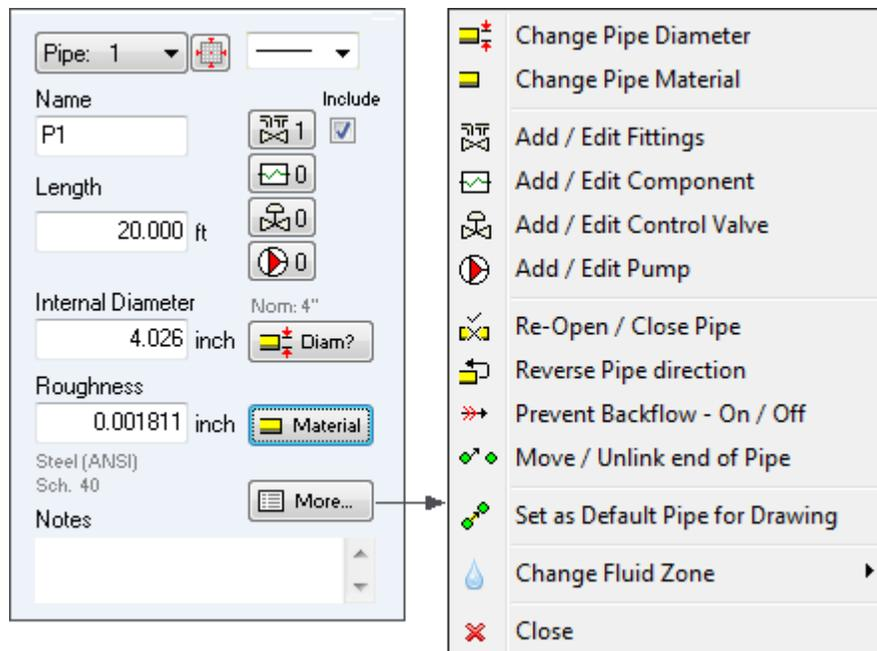
Figure 17 Pipe Pane and Pipe Sub-menu
