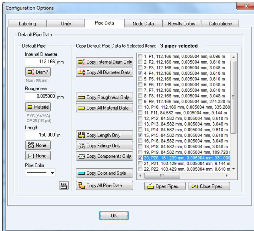
Figure 37 Configuration Options – Pipe Settings tab
