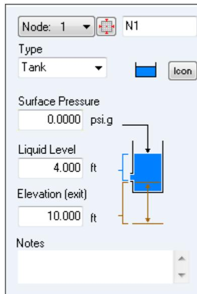
Figure 48 Node Pane for Tanks
