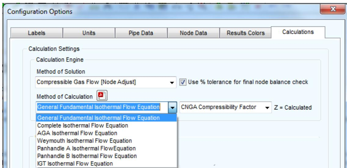
Figure 99 Compressible Flow Calculation Options
