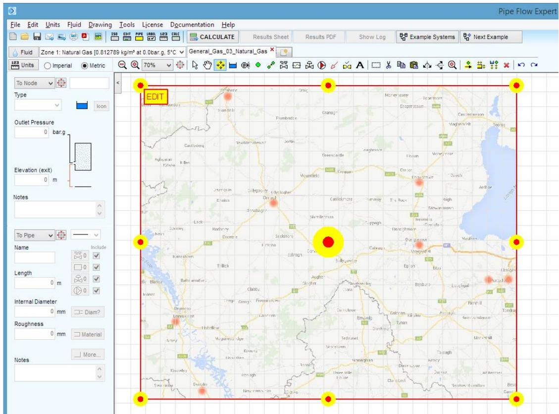
Figure 76 Importing an image on to the drawing
