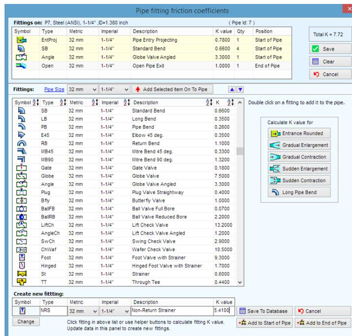
Figure 55 Add a fitting in the Pipe fitting friction coefficients listings
