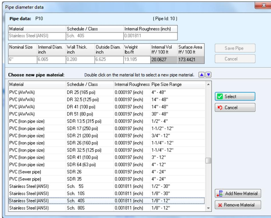
Figure 51 Pipe diameter data - materials list
