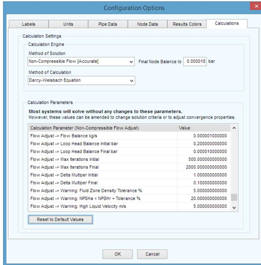
Figure 30 Configuration Options - Calculations Tab
