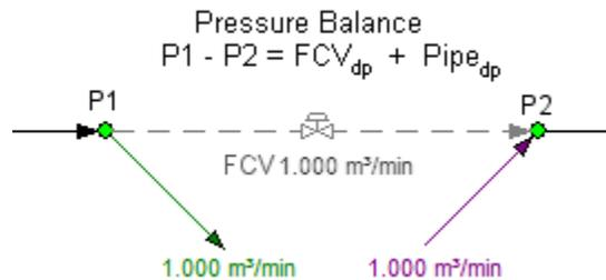
Figure 95 Flow Control Valve replacement
