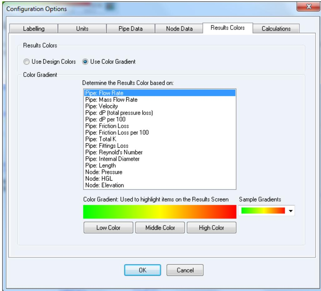
Figure 29 Configuration Options - Results Colors tab
