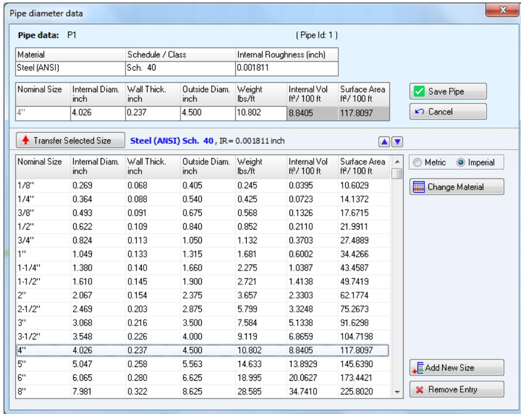
Figure 19 Pipe Diameter Data
