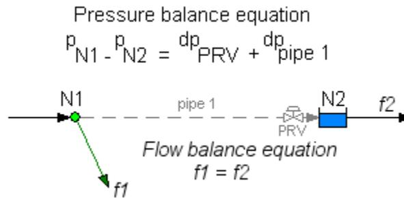
Figure 96 Pressure Reducing Valve replacement
