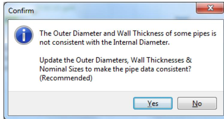
Where an Internal Diameter has been amended by over typing the data in the pipe pane or the edit grid the Outer Diameter, Wall Thickness & Internal Diameter may no longer be consistent with each other.
