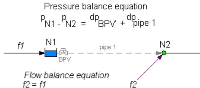
Figure 97 Back Pressure Valve replacement
