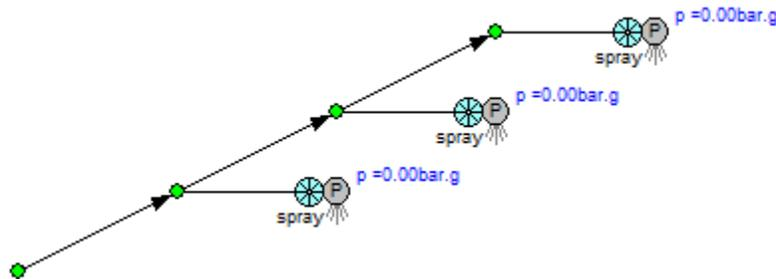
Figure 62 Modeling a Spray Nozzle
