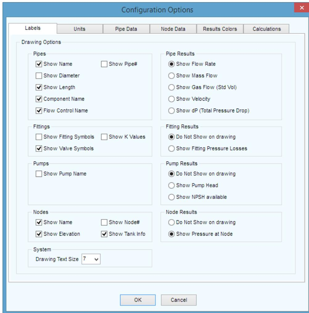
Figure 84 Configuration Options dialog – Labelling tab
